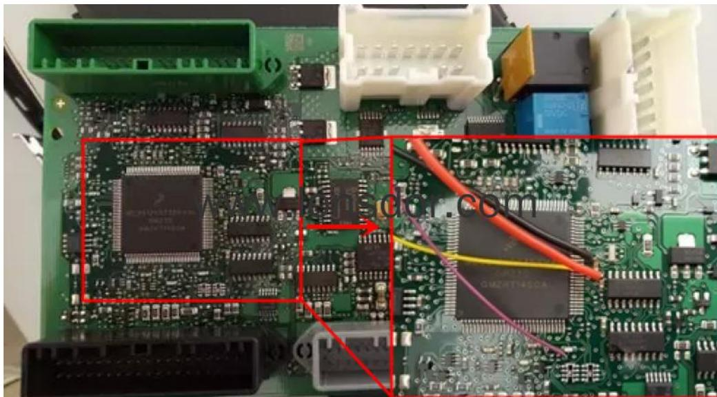
Read the bin file, import it into K518: Please use the USB cable to connect K518ISE with computer, open the device internal memory, find the folder "customfile" and put BIN file into it.
